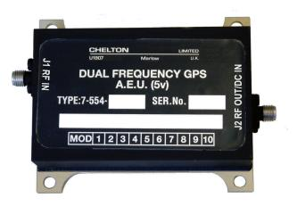
The pre-amplifiers are supplied configured to provide factory set gain that ranges from 12 dB to 24 dB.
